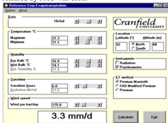
Fig 1. The program (software) used to apply the formulae Penman-Monteith
